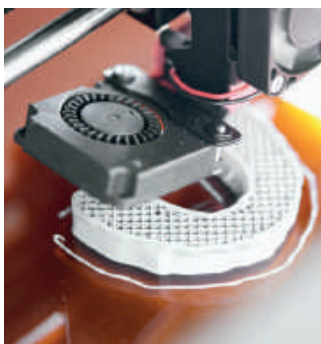
Fig. 3 Filament printing (FDM/FFF procedure)
