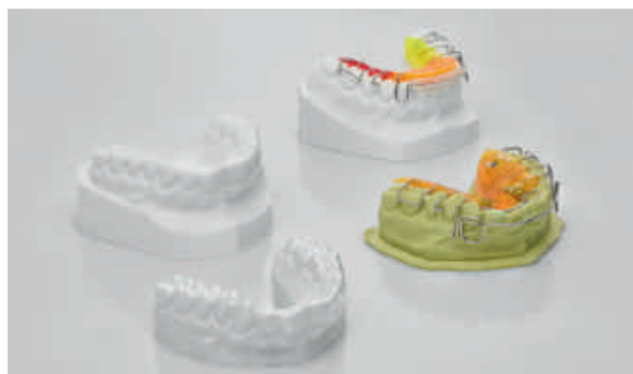
Fig. 4 Finished orthodontic models directly after printing
