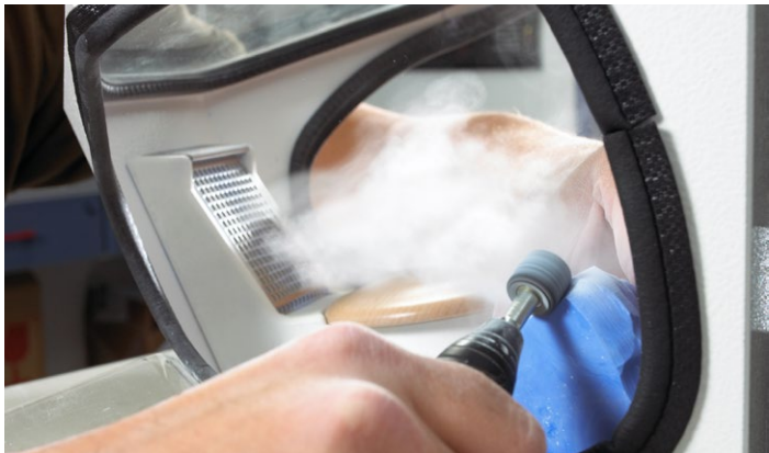
In the case of particularly large amounts of dust, the Dustex master plus dust extractor box keeps the workbench clean.
