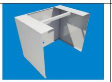
Insert **HORIZONTAL BAR** near top front in "L" shape as shown in photo (to SQUARE the box)
