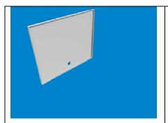
Ensure REAR WALL has flanges towards you (front) and 1.5"diameter hole on bottom
