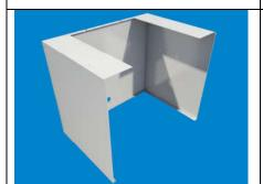
Place <u>LEFT SIDE WALL</u> at 90 degrees from **REAR WALL**, ensure LEFT SIDE WALL flanges are towards RIGHT, Fasten together using <u>3 screws</u>, <u>DO NOT TIGHTEN</u>
