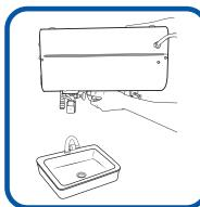
Turn the unit upside down to drain all the water in the tank. Add clean water and repeat if necessary to remove any sediment.
