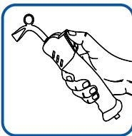
Press the steam button on the steam handle until the pressure drops to zero.
