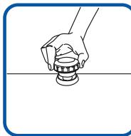
Open the filler safety cap slightly to allow the remaining steam to release.
