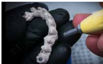
Sandblast framework with Al 2 O 3 (50µm, 0.2MPa)
