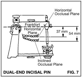
The Incisal Pin is inserted into, and the wider mid-line of these metric grooves is aligned with, the top edge of the Upper Member. It is secured by the Thumbscrew bearing against the flatted side on the Pin. This adjustment places the chisel end at 90 degrees to and in contact with the central table of the Incisal Guide and provides a parallelism of the Upper Member to the Lower Member.
