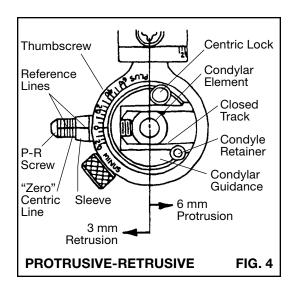
An axial reference line transcribes the one mm spaced lines on the P-R Screw and a like line appears on the Sleeve of the Guidance.
