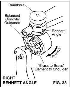
41. While still maintaining this lateral position in the record, slightly loosen the Thumbnut for condylar inclination, Figure 32, and reaffirm the record seating by slightly rotating back and forth, then retightening the Thumbnut.
