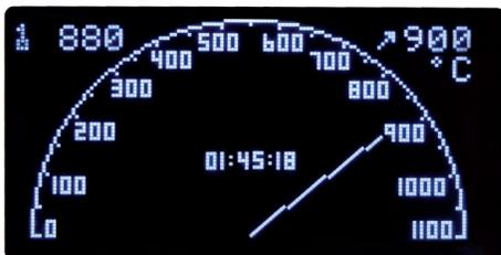
The hold countdown continues to count down even though the temperature decreases after opening the muffle door.
