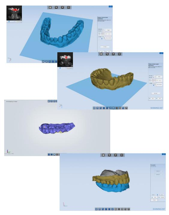
To design the splint, I used **Exocad's Splint** and **Virtual Articulator** modules. The latter allows to mount the case on a virtual articulator of your choice, in this case, a Panadent PCH, and perform the jaw movements to insure the prescribed guidance.
