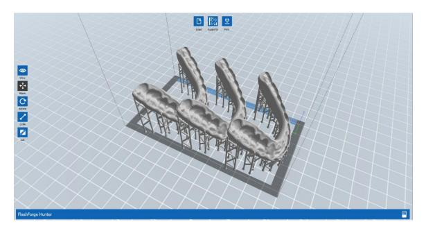
At 100um layer thickness, this layout took 1 hours and 20 minutes to print, using the Hunter's Fast mode. Yes, the Hunter can print at 50um or 25um layer thickness, but for a splint, there's no real need for that since there isn't any fine detail. Reducing the layer thickness in this case
