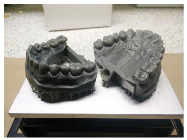
To test the difference in the adaptation, I also poured a set of models in dental stone. My initial prediction was that, since 3D printable resin shrinks a bit and dental stone expands, the splint would fit snuggly in my mouth, fit perfectly on the printed model and fit too tightly on the stone model. Was I right? We'll find out soon enough.
