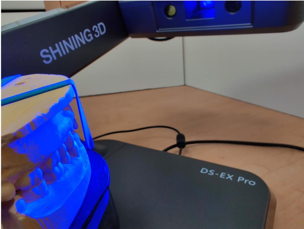
I was particularly impressed with its ability with uncut models. One particular model which gave me some grief in the past with the lower end DS-EX was a Geller type I made some time ago. The trenches around each preps are deep and sharp. Previously, with the DS-EX, I would end up with voids around the die margins. With the DS-EX Pro H, and Multi-path scanning enabled, it scanned this model in one shot, with no voids!
