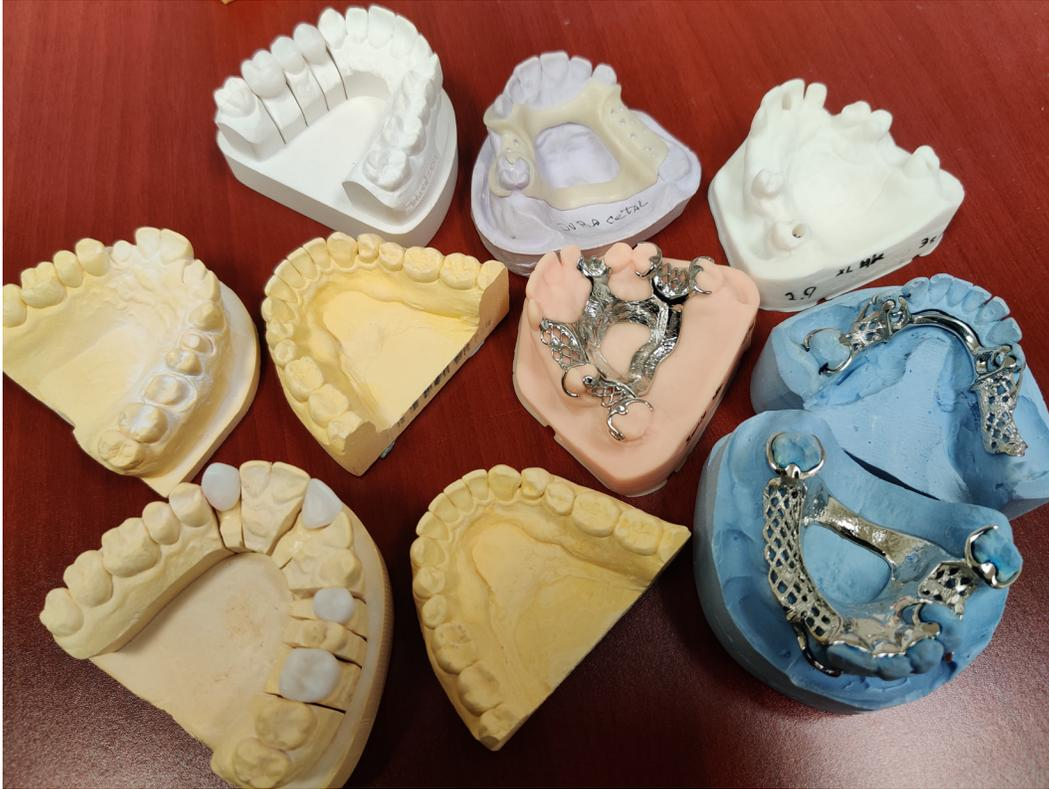
The method would consist of scanning the models, print them out and test fit the restorations and frameworks on them.
