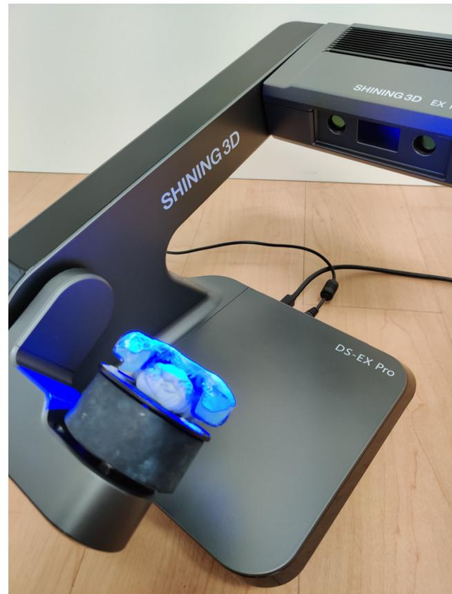
Once again, the DS-EX Pro H doesn't disappoint. After a single pass, the impressions are practically whole, with a few minor voids which DentalScan's Intelligent and Manual Add-Scan functions handle with ease.
