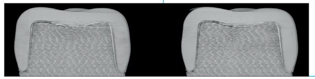
Fig. 11: Comparative μCT image (sectional view) of a cemented crown before (left) and after (right) the chewing simulation
