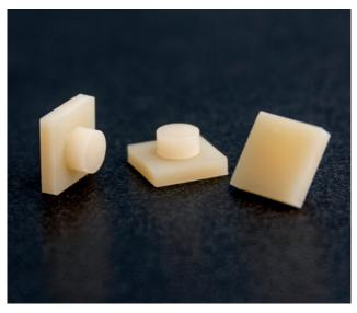
Fig. 13: Test specimen for determination of bond strength
