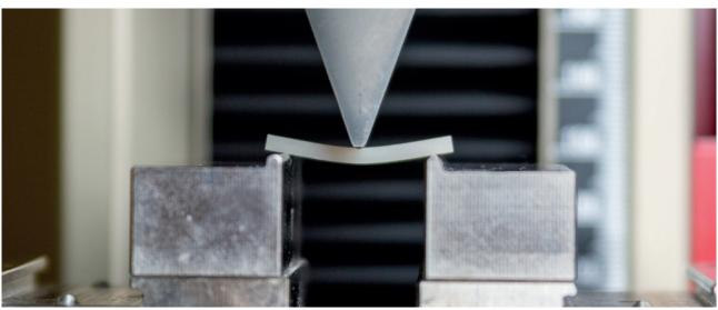
Fig. 14: Determination of the flexural strength
