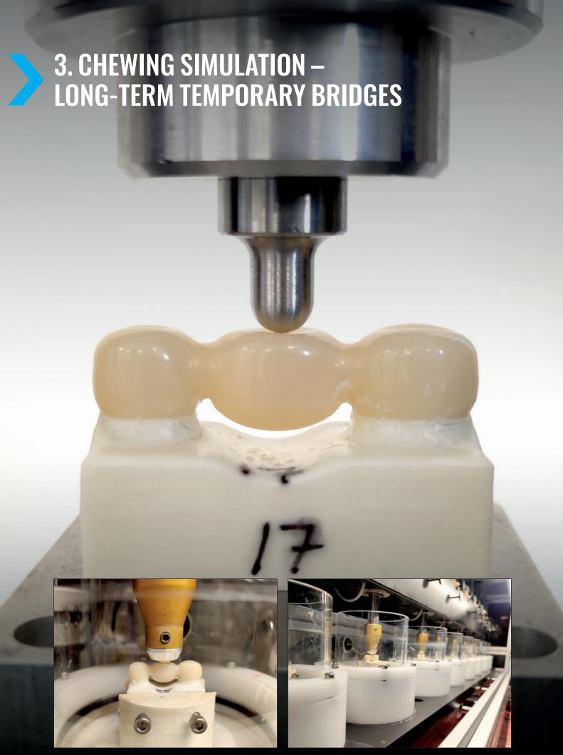
Fig. 6 and 7: Experimental setup of the chewing simulation for long-term temporary bridges
