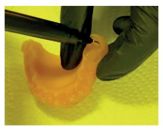
Fig. 15: Application of the liquid FREEPRINT® DENTURE material into the cavities under yellow light
