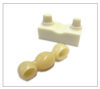
Fig. 8: Test specimen geometry for the chewing simulation
