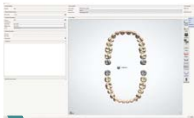
1 Create case and mark teeth to be replaced; Type: Artificial Tooth Type; Material: VITA VIONIC VIGO Artificial Teeth; Manufacturing Process: Milling VITA VIONIC BASE.
