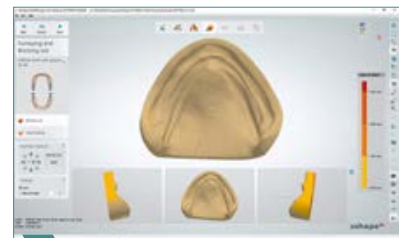
9 Define the insertion direction. Pay attention to undercuts.
