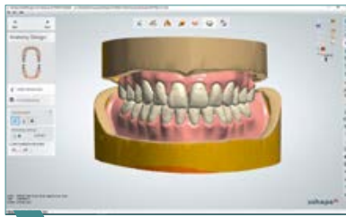
13 The Sculpt toolkit is used to modify the gingiva morphology.
