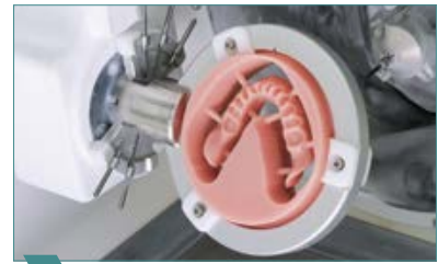
3 Mill the final mandible denture base.
