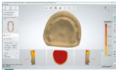
7 Define the insertion direction. Pay attention to undercuts.
