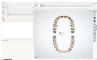
2 Create denture gingiva; Type: VITA VIONIC BASE with artificial teeth; Material: VITA VIONIC BASE HI; Manufacturing Process: Milling VITA VIONIC BASE.
