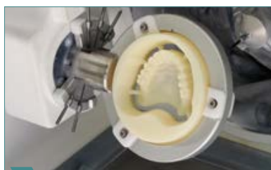
2 Mill the wax disc for the full-sized wax try-in (here: UJ).
