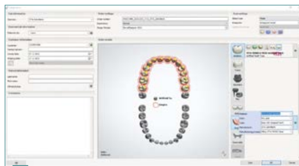
➤ 2 Create gingiva: Type: Base with designed teeth; Material: VITA VIONIC BASE HI. Manufacturing process: Milling VITA VIONIC BASE.
