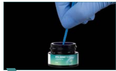
3 Mix the two components for 30 seconds to prevent air bubbles.
